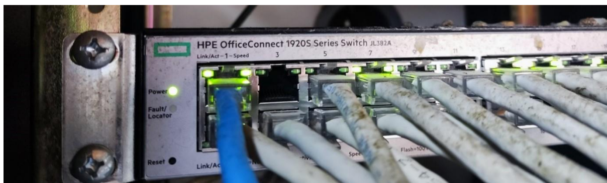
Figura 12: Switch HPE OfficeConnect 1920S Series
